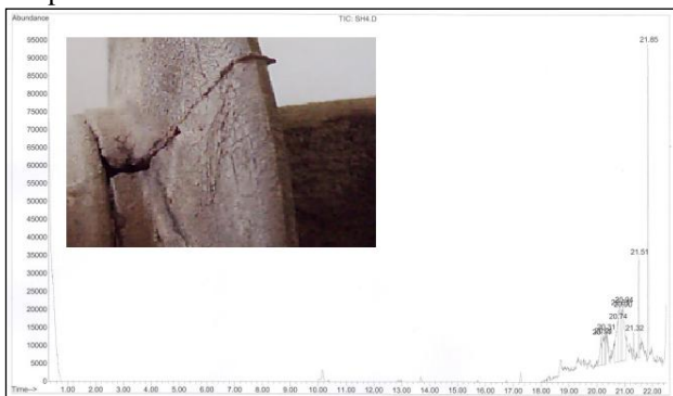
Fig8: gas chromatograms for composite insulator sample from level 5
