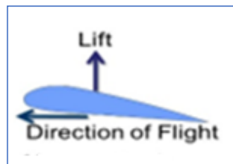
Figure 1: Lift force and its effect on the motion of the blades
